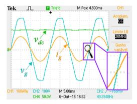
Figure 5: Experimental results of the symmetrical bridgeless topology: Power grid voltage (vg); Dc-link voltage (vdc); Grid current (ig).
