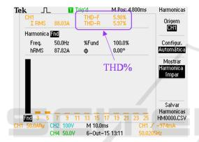
Figure 8: Experimental results of the asymmetrical bridgeless topology: Harmonic spectrum of the grid current and measured THD%.
