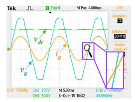
Figure 3: Experimental results of the traditional power factor correction topology: Power grid voltage  $(v_g)$ ; Dc-link voltage  $(v_{dc})$ ; Grid current  $(i_g)$ .
