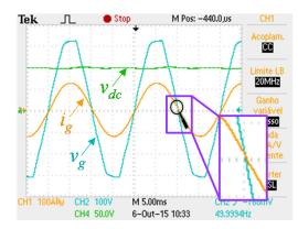
Figure 9: Experimental results of the full-bridge full-controlled topology: Power grid voltage (vg); De-link voltage (vdc); Grid current (ig).
