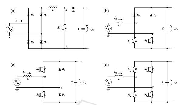
Figure 1: Single-phase active rectifiers under comparison: (a) Traditional power-factor-correction (PFC); (b) Symmetrical bridgeless; (c) Asymmetrical bridgeless; (d) Full-bridge full-controlled.
