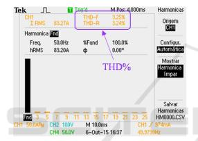
Figure 4: Experimental results of the traditional power factor correction topology: Harmonic spectrum of the grid current and measured THD%.
