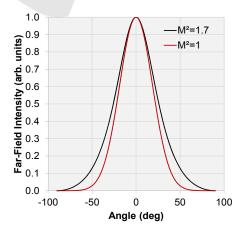
Figure 6: Near-field (left) and far-field (right) intensity distributions for an engineered structure with M<sup>2</sup> of 1.7 and 86 percent of its power in the far-field within the diffraction limit.
