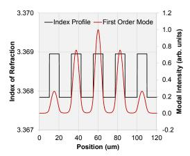
Figure 2: A structure useful for demonstrating the effects of changes to the index profile.
