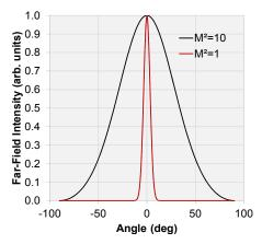
Figure 7: Near-field (left) and far-field (right) intensity distributions of an engineered structure operating with M<sup>2</sup> of 10 and only 20% of its power in the far-field within the diffraction limit.
