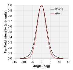
Figure 9: Near-field (left) and far-field (right) intensity distributions of an engineered structure operating with M<sup>2</sup> of 19 and 89% of its power in the far-field within the diffraction limit.
