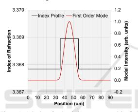
Figure 1: A basic refractive index structure and its first order mode profile. Note that many higher order modes are also supported by this structure.
