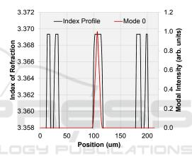
Figure 8: The index profile and first order mode of the engineered structure that supports the original hypothesis.
