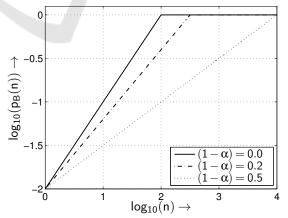
Figure 6: Approximated block buyer's probability  $p_{\rm B}(n)$  as a function of the interval length *n* for different parameters of the  $(1 - \alpha)$  at a buyer's probability of  $p_{\rm e} = 10^{-2}$
