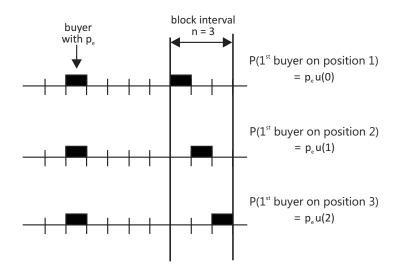
Figure 7: Calculating the block-error probability  $p_{\rm B}(n)$  using the error-gap distribution function u(k)
