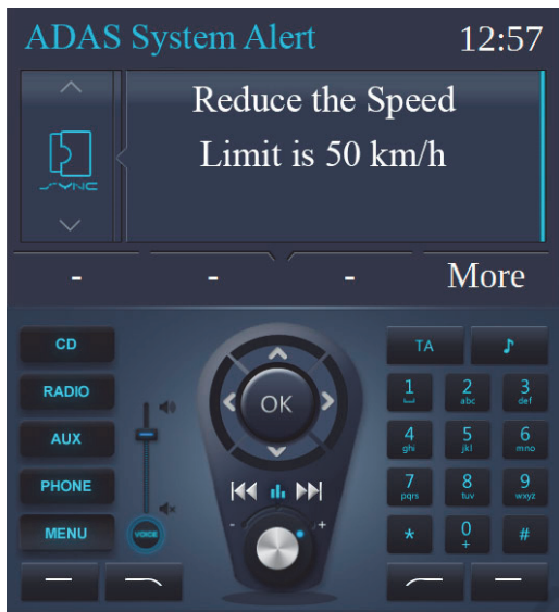
Figure 5: Example of Smartphone ADAS system integration with Ford Sync.
