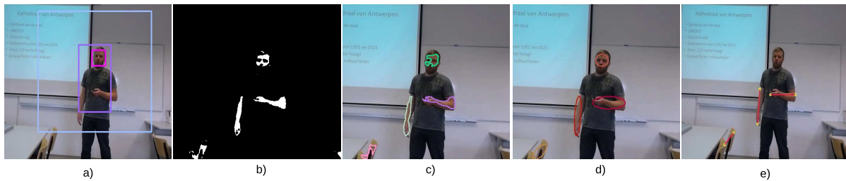
Figure 3: Generation of hand candidates: a) original image, b) skin segmentation, c) contour detection, d) fit ellipse, e) final hand candidates.
