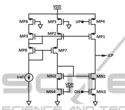
Figure 6: Transistor level implementation of charge pump.
