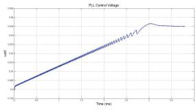
Figure 11: PLL control voltage.
