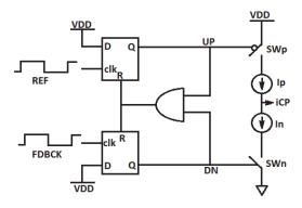
Figure 5: PFD along with charge pump configuration.
