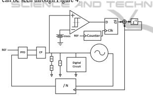
Figure 3: Proposed architecture for control voltage setting.
