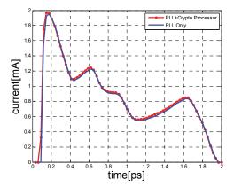
Figure 14: PLL supply current before and after adding the crypto-processor.
