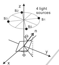
Figure 3: Geometry of quadrature phase light sources and surface normal.
