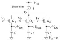
Figure 2: Pixel structure of the correlation image sensor.
