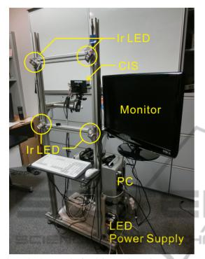
Figure 4: Photograph of real time surface orientation imaging system.
