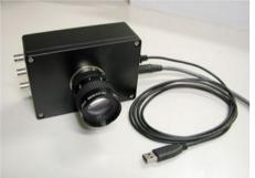
Figure 1: Photograph of Correlation Image Sensor(CIS).
