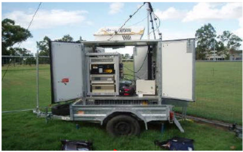
Figure 3: Mobile station for monitoring the air.
