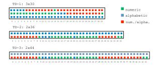
Figure 5: Structure of Machine-Readable Zones. There are three different types, which contain two or three lines of text. This corresponds to 90, 72 or 88 individual characters.
