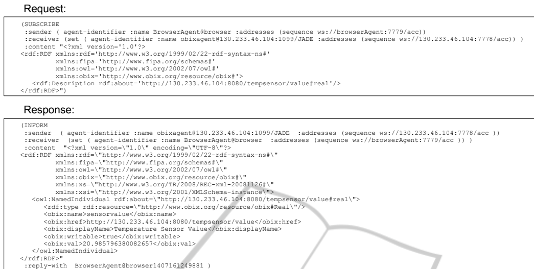
Figure 4: A subscription request from a browser agent to the gateway agent and a response sent by the gateway agent.
