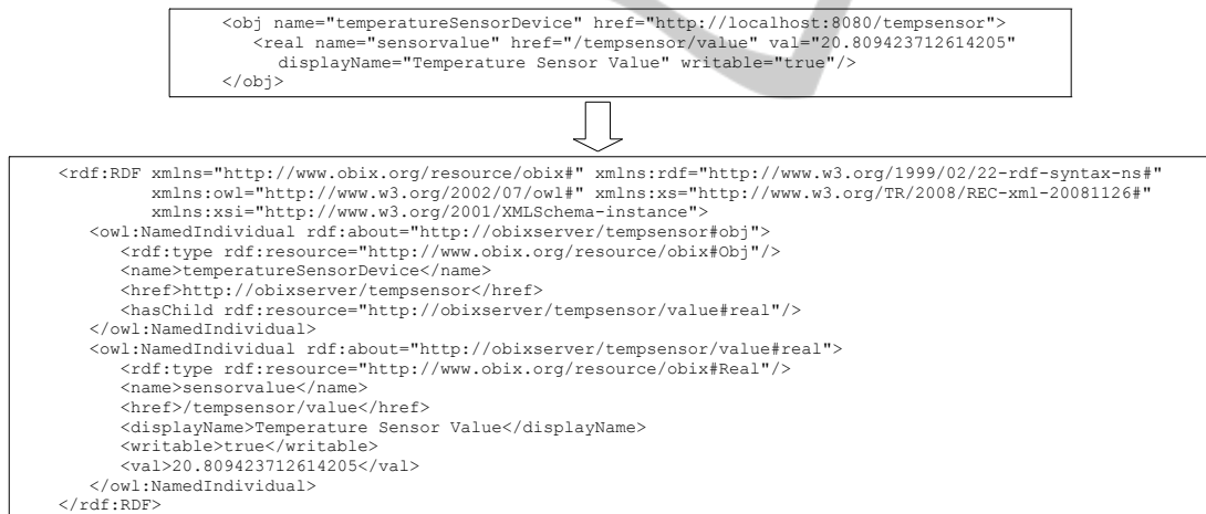
Figure 3: An example transformation from oBIX XML to RDF/OWL.
