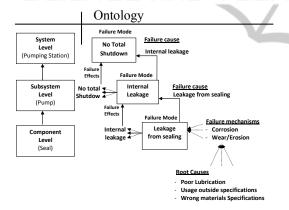
Figure 6: The relationship between failure cause, failure mode and failure effect. (Adapted from Source: (Rausand and Høyland, 2004).
