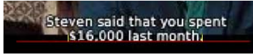
Figure 6: Example of a frame where the subtitle intercepts the active image area boundary; in this case, only three subtitle limits will be found.
