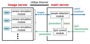
Figure 5: Structure of the prototype system.
