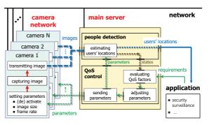
Figure 3: Structure of the proposed QoS control method for camera network based people detection systems.
