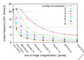
Figure 7: Output frequency (OF) by varying the number of cameras and the size of image.
