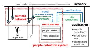
Figure 1: Supposed configuration of a people detection system based on a camera network.
