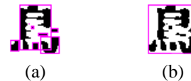
Figure 6: (a) A Kanji character divided with several rectangles, (b) A Kanji character surrounded by one.
