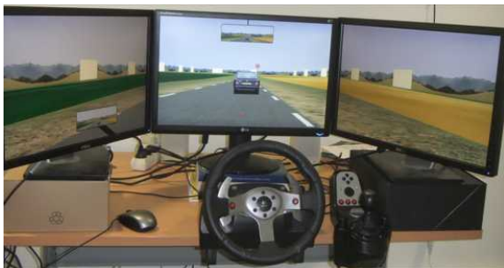
Figure 2: Driving simulator device with 3 screens, steering wheel, gearbox and a set of pedals.
