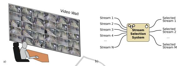
Figure 1: a) An operator in front of a video wall. b) Stream selection task: at any time instant, select the M streams, among N, that are the most meaningful to show to a human operator.
