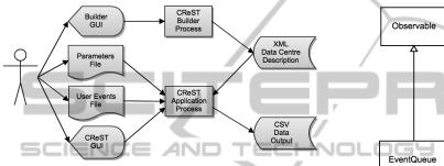
Figure 1: CReST architecture diagram.
