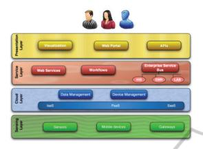
Figure 1: SOA & Cloud based Architecture for Non-Invasive Health Monitoring.
