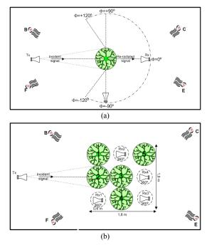
Figure 1: Measurement geometry of the: a) single tree and b) tree formation scenarios.
