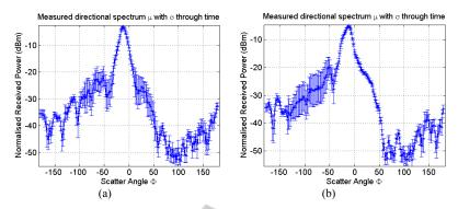
Figure 6: Measured directional spectrum from position Rx2, with wind incidence from: a) B and b) F.
