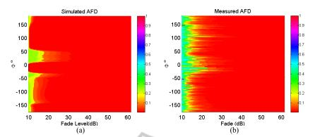
Figure 14: Comparison of data from position Rx2, with wind incidence E, between: a) simulated and b) measured data sets.
