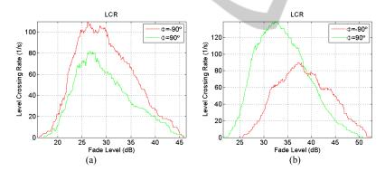
Figure 4: Measured LCR statistics at  $\Phi$ =-90° and  $\Phi$ =90°, for wind incidences from: a) B and b) F.
