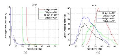
Figure 5: Measured statistics at  $\Phi$ =-90° and  $\Phi$ =90°, for wind incidences from B and C, concerning: a) AFD and b) LCR.
