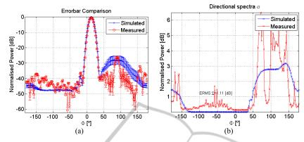
Figure 11: Comparison between measured and simulated data from position Rx1, with wind incidence C, considering: a) directional spectra errorbar and b) directional spectra standard deviation.
