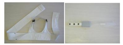
Fig. 5. Textile enclosure and device for chest use.
