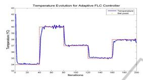
Figure 7: Control evolution with adaptive FLC algorithm for various set points.
