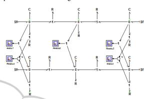
Figure 8: DBG of the three tanks system.
