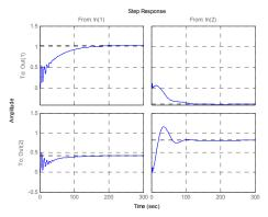
Figure 5: Step response of closed-loop with Controller.
