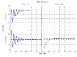
Figure 3: Step response without Controller.
