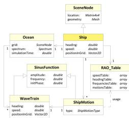
Figure 6: UML Class Diagram of the Ship.
