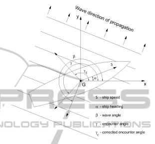
Figure 3: The encounter angle is given by the difference between the wave angle and the ship heading.
