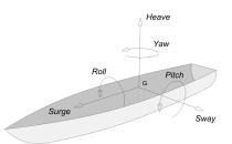
Figure 1: Ship motion is divided into six components in the six degrees of freedom.
