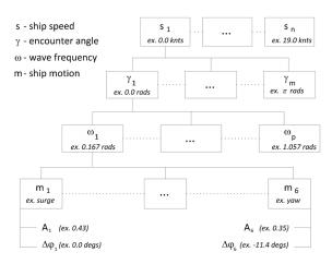
Figure 4: RAOs values are read from ASCII files and stored in hierarchical tables.
