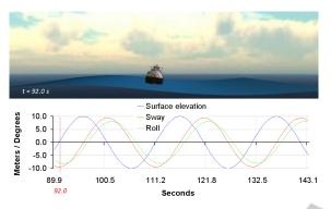
Figure 11: Ship subjected to a single wave train coming from starboard with amplitude of 10.0 m, frequency equal to 0.310 rad/s and wavelength of 640 m.
