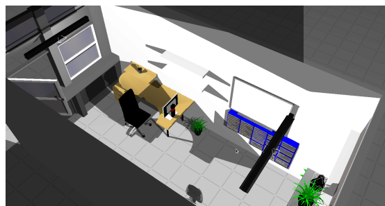
Figure 1: The Cognitive Office , our intelligent cognitive environment in 3D simulation. Physical objects like drawers, windows, doors and plants and corresponding events are linked to their virtual representations in real-time.
