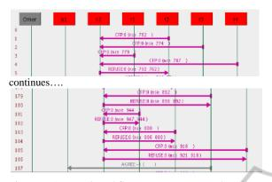
Figure 5: A normal workflow announcement to the *Alarm Agent* using JADE Sniffer tool.
