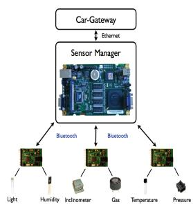
Figure 2: General architecture of the sensor network.
