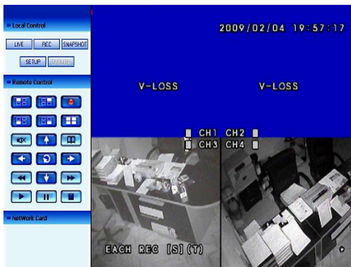
Figure 1: Live view module, a system using a DVD and IR cameras.
