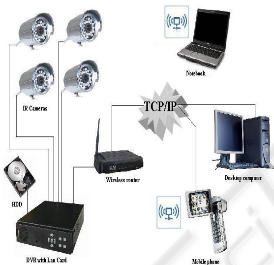
Figure 4: Video surveillance/monitoring system using DVD.
