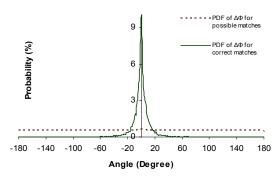
Figure 4: The experimental PDF of the angle difference for the incorrect and the possible matches.
