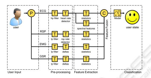
**Fig. 4.** State flow of the online emotion recognition component developed with SSI as part of the METABO project: each sensor channel is first processed individually before features are finally combined to a single feature vector. The combined feature vector is analyzed by the recognition module.
