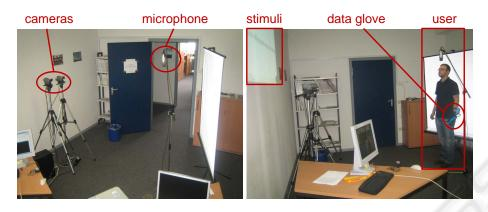
**Fig. 2.** The Figure shows the setting of an affective gesture recognition experiment carried out in the CALLAS project. Users are recorded from two cameras, one microphone, and additional interaction devices such a data glove.
