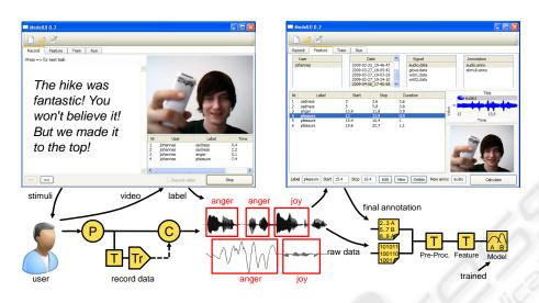
**Fig. 3.** The Figure shows two screenshots of the graphical interface we have developed on top of SSI. It helps the experimenter to record the user interaction (left image) and let him review and annotate the recordings (right image). It also leads through the other steps of the training procedure. The GUI uses a DLL to communicate with SSI (see sketches below the screenshots).
