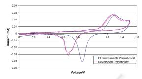
Figure 5: Cyclic Voltammogram for the developed potentiostat and a CHInstruments Potentiostat in 0.5M H2S04.
