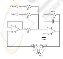
Figure 3: Potentiostat sensor control circuit with input stimulus voltage from DAC and connections to sensor.
