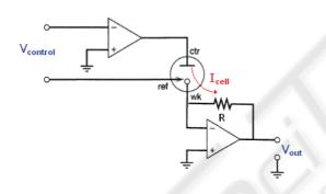
Figure 1: Standard potentiostat topology with inverting control amplifier and transimpedance current measurement.
