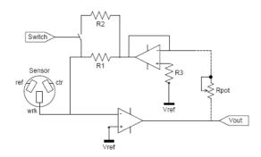
Figure 4: Transimpedance amplifier circuitry for measurement of working electrode current including external digital potentiometer.
