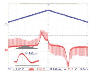
Figure 6: Time domain potentiostat response to a DAC generated cyclic voltammetry signal.
