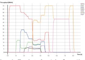
Figure 1: Throughput of particular flows without utilization of QoS mechanisms.
