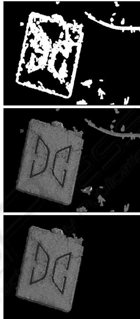
Figure 4: Binary dilation with a circular structuring element is applied (top). After region growing (middle), objects which do not meet the expected size are removed (bottom).
