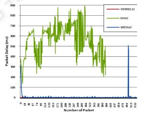
Figure 2: Comparison of Packet delivery delay in different MAC protocols for  $6 \times 2$  grid deployment.
