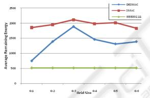
Figure 4: Average network remaining energy for different network sizes.
