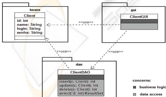
Figure 3: Class diagram of the three layer implementation of the application.
