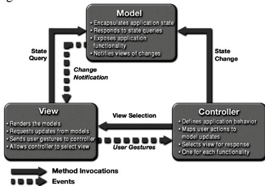
Figure 2: The Model-View-Controller design pattern.
