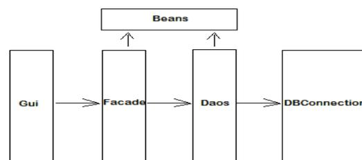
Figure 1: The proposed software architecture model.
