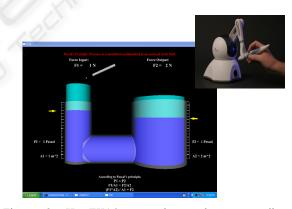
Figure 8: HaptEK16 screenshot and corresponding Phantom<sup>™</sup> device from Sensable Technologies.
