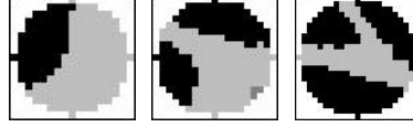
Fig. 7. Visualization of junction templates: E_{r_1} contains the adjacent cells in black. The information of the veins is derived from the extruded cells (dilation with a circle, marked in light gray). Pixels outside of these extruded cells are unknown and marked in dark gray. The examples show (f.l.t.r.) one, two or three adjacent cells. Thereby, the values of the radii (f.l.t.r. 17, 19 and 23 [pxl]) are chosen by the taxonomic expert and encode the expert knowledge about the relevant local feature neighbourhood for placing the junctions.
