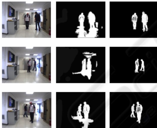
Figure 4: The figure shows the results obtained by motion detection and shadow removing algorithms on images acquired in a laboratory.
