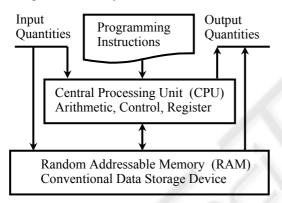
Figure 1: Programmed data processing computer
