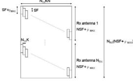
Figure 1 : Layout of the SCA matrix
