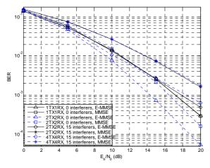
Figure 9 : E-MMSE vs MMSE scheme – QPSK modulation, Pedestrian A channel
