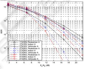
Figure 7 : E-MMSE scheme – 16QAM modulation, 0 interferers
