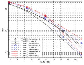
Figure 8 : E-MMSE scheme – 16QAM modulation, 15 interferers
