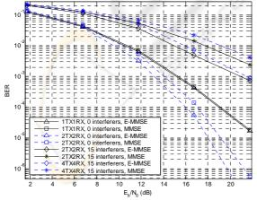
Figure 11 : E-MMSE vs MMSE scheme – 16QAM modulation, Vehicular A channel
