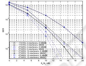
Figure 10 : E-MMSE vs MMSE scheme – QPSK modulation, Vehicular A channel
