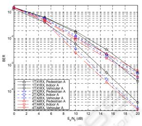
Figure 6 : E-MMSE scheme – QPSK modulation, 15 interferers
