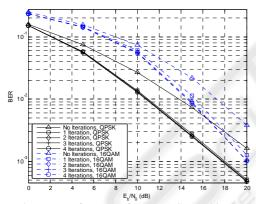
Figure 4 : BER performance for E-MMSE, Vehicular A channel, MIMO 2x2, 15 interferers - effect on number of cancelling stages.
