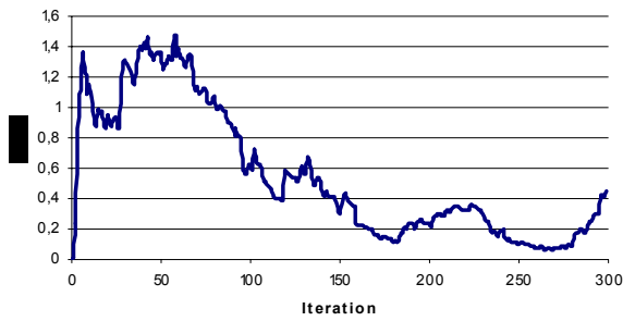
Figure 4: Evolution of the mean squared error between the output of the world model (distance to the object) and the real distance.
