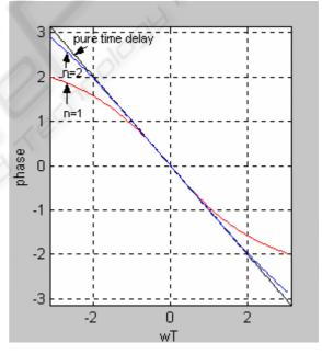
Figure 1: Phase-frequency characteristics of time delay block and Pade's functions
