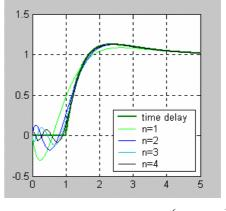
Figure 8: Plant  $G(s) = e^{-\tau s} \frac{K}{T_1 s + 1} \left( 1 + \frac{T_d s}{Ts + 1} \right),$  $(T_1 T/T_d \approx \tau)$
