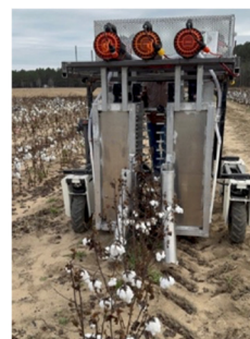
Figure 9: Harvester robot positioned to harvest cotton bolls from the treatment row.
