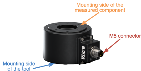
Figure 6: BOTA Systems Medusa force/torque sensor.
