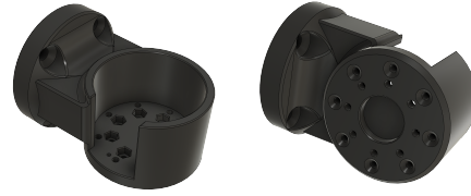
(a) Top view (b) Bottom view Figure 7: Second force/torque sensor adapter.
