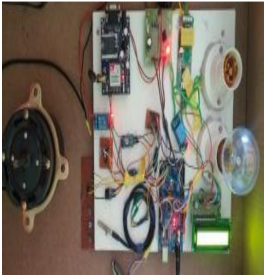
Figure 8: IoT-Based Smart Energy Monitoring and Control Prototype.
