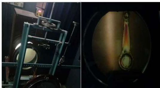
Figure 4: (left) Experimental setup and (right) Tensile and compressive loads acting from both ends.
