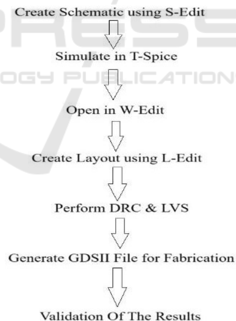
Figure 2: Algorithm of proposed 4-bit nano processor using TG.
