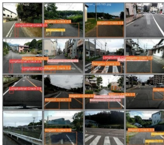
Figure 3: Sample Annotated Images from the Road Defect Dataset Showing Various Types of Cracks Such As Longitudinal Cracks, Alligator Cracks, and Transverse Cracks Used for Training and Evaluation.
