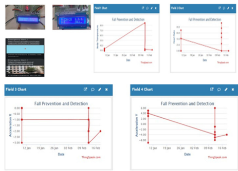
Figure 3: The implementation and data visualization of the fall prevention and detection system. It includes hardware setup with LCD displays (a) and real-time monitoring graphs for body temperature, heart rate, and acceleration in X and Y axes (b – e) using ThinkSpeak. These visualizations help in analyzing fall patterns and system
