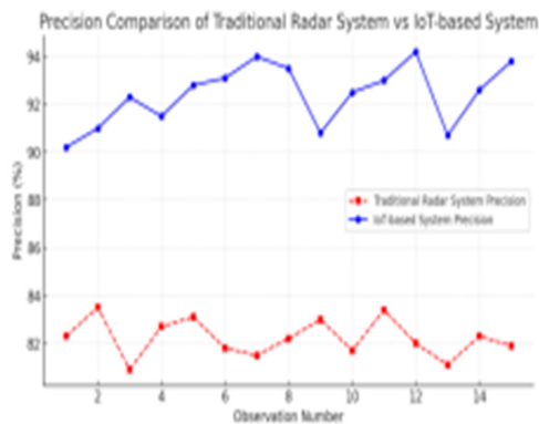
Figure 3: Precision Comparison of IoT-Based System (ESP32) and Traditional Radar System Across Observations.
